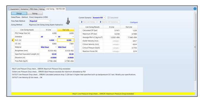
Based on calculation, the pressure drop for both inlet and outlet has exceeded the criteria. In order to resolve the issue, let's select a line with bigger size for inlet and outlet.
