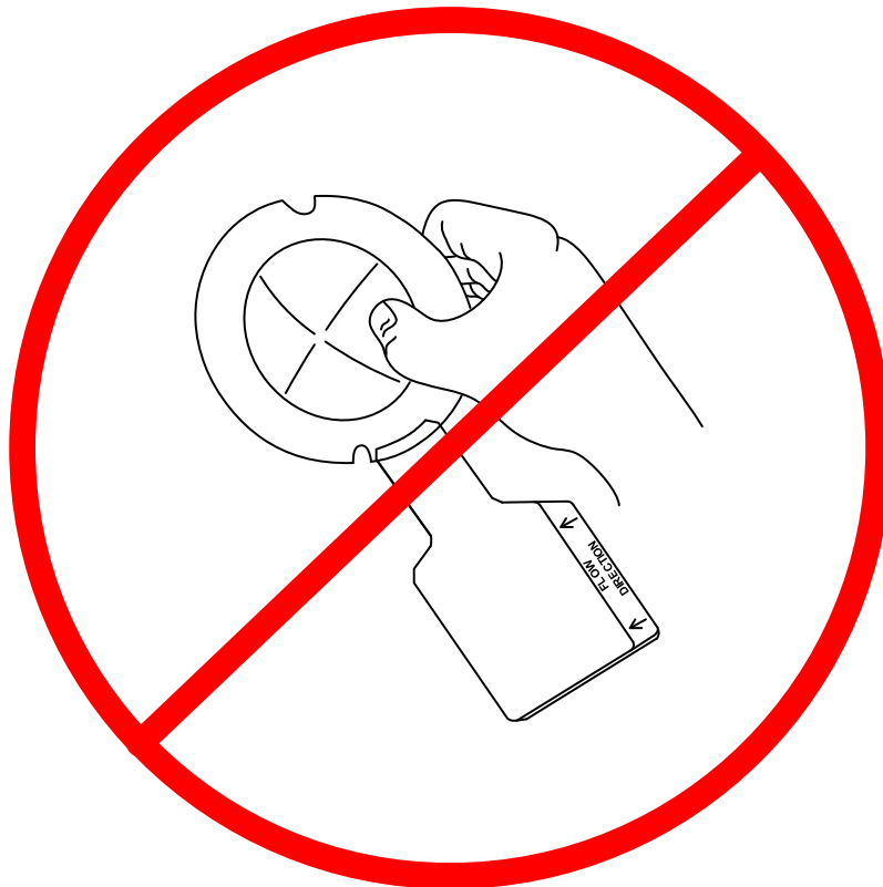
Figure A.3—Improper Handling of a Rupture Disk
