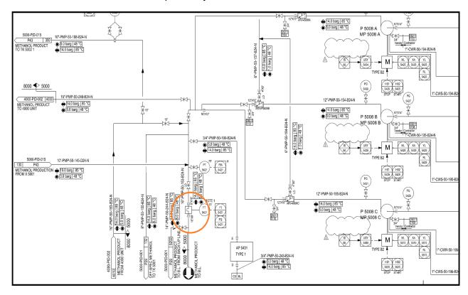
Since the flowmeter is used for product, we then use Coriolis flowmeter.
