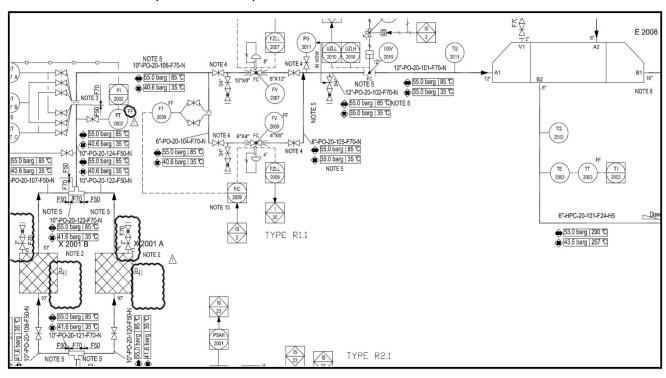
The size of the line is 10" and design temperature and pressure are 85C and 55 barg, respectively.
