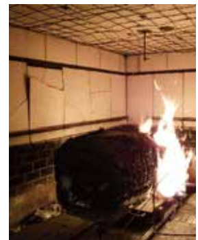
SchuF Globe Valve being fire-tested [Fire-safe Certification available, e.g. API 607]
