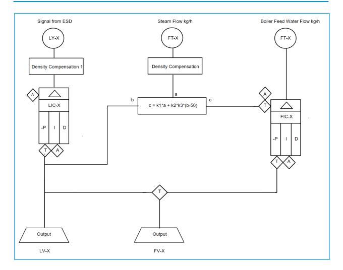
Remember the density compensation 1 is different from density compensation for saturated steam flow.
