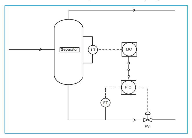
The controller driving the set point (the level controller in the example above) is called the primary, outer, or master controller. The controller receiving the set point (flow controller in the example) is called the secondary, inner or slave controller.
