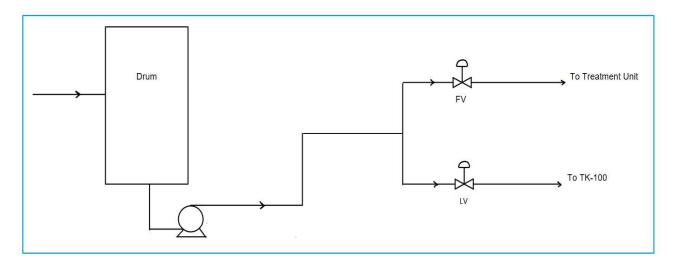
Simply the blow-down is sent to a treatment facility outside of the plant. Based on PFD-like sketch, the flow to treatment unit is controlled via FV while the flow to TK-100 is controlled by LV. Sometimes the treatment unit is out of service for say half a day and thus, cannot receive the blow-down. Therefore, the process designer should foresee a storage tank to overcome such operational problems in the future.
