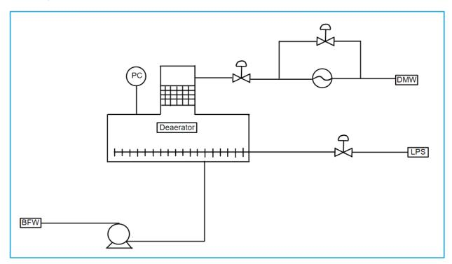
You see the aim of the deaerator is to eliminate oxygen mechanically. So far, we have talked about packed bed, which increases the mass transfer between exiting steam and DMW; we also talked about LPS injection, which un-trap the trapped oxygen molecules. Here are more initiatives to apply in deaerators to help remove the oxygen.
