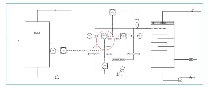
Everything is in order except the FHIC controller part, which is shared by both Master controllers FIC and LIC. It is abnormal that the controller receives two MV at the same time; it is meaningless and the controller becomes confused which MV to take.
