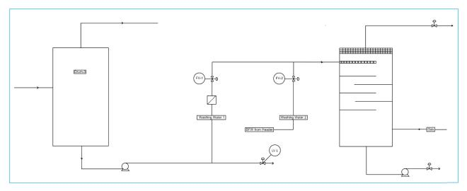
The aim here is to always maintain and keep washing water flowrate within the range. So we need a FIC for this purpose; it is also crystal clear that we should have split-range control since the controller should operate two control valves.
