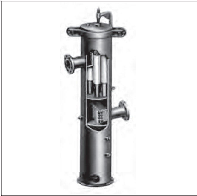
FIG. 7-46 Vertical Filter Separators
