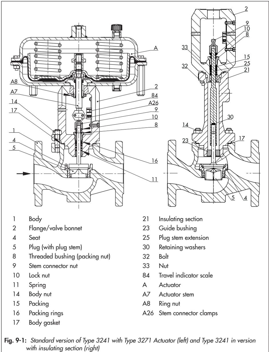
**Fig. 9-1:** Standard version of Type 3241 with Type 3271 Actuator (left) and Type 3241 in version with insulating section (right)
