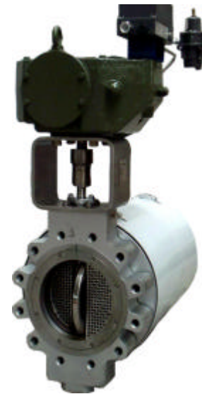
Fig. 1 · Control Butterfly Valve Type LDE (with LN and Diffuser) with diaphragm Actuator and E/P Positioner
