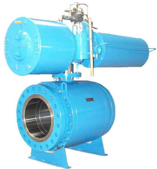
Fig. 1 · High pressure Ball Valve Type SE 16" ANSI 900, with pneum. spring return Actuator and E/P Positioner
