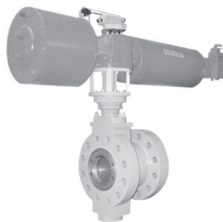
Fig. 1 · Type LTR 43 High-pressure Butterfly Valve in double flange version, size 10", ANSI Class 1500 with pneumatic actuator and positioner
