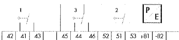
1 pilot valve 3 electric contacts (change-over contacts)
