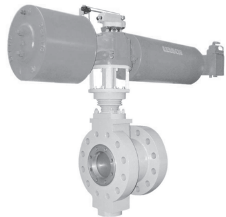
Fig. 1 · Type LTR 43 High-pressure Butterfly Valve in double flange version, size 10", ANSI Class 1500 with pneumatic actuator and positioner
