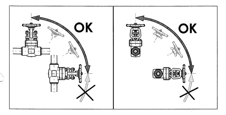
These valves should be installed, where it's possible, on horizontal line, with the stem upwards. It is accepted that a position between vertical and horizontal guarantees a correct drainage.
