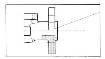
Before the assembly, make you sure that the flanges valve/line are JK of the same type or, in any case, complementary.
