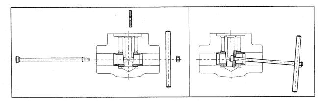
Disks can be polished on every plane surface, but trying to keep the correct wedge (10° at the axis).
