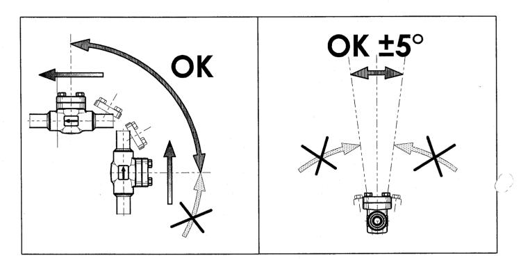
These valves too should be put along horizontal lines with cover towards the up side.
