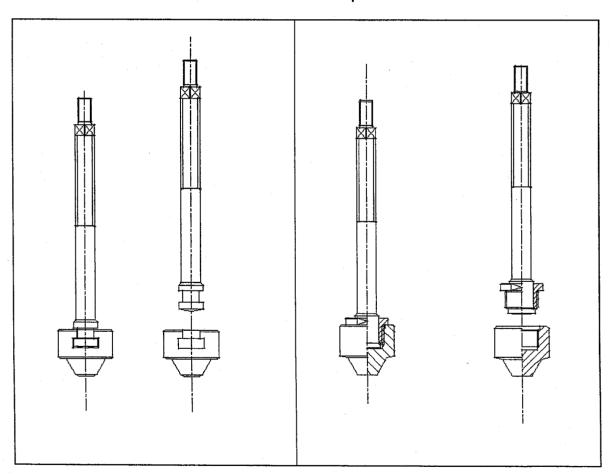
In ball and piston check valves the damaged disk can be easily taken off to be replaced.
