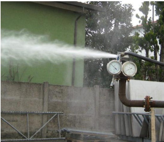
Narrow spray pattern for probe mounting
