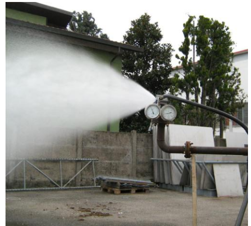
Wide spray pattern for side wall mounting
