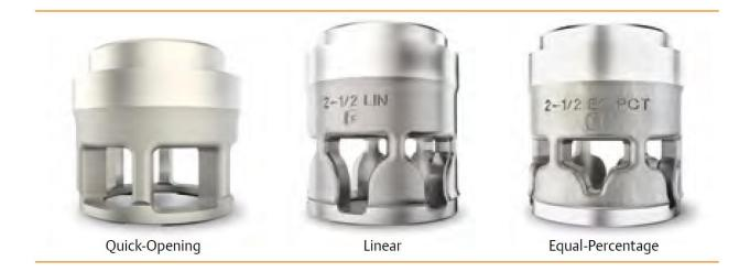
Even though based on above rules a linear characteristic should be selected for pressure applications, an equal-percentage is selected due to start-up conditions in which at first stages of start-up low opening of the valve is required while at normal condition high opening is demanded. Equal percentage characteristic fulfills such demand and therefore is selected.
