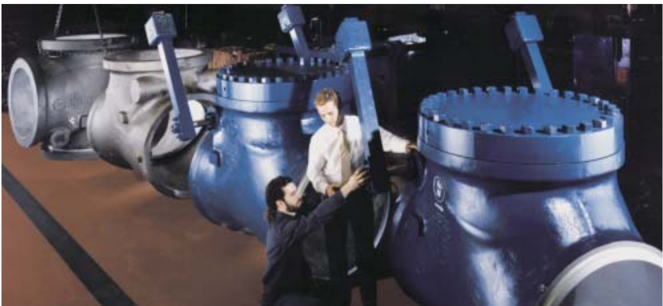
44" Cold Reheat Check Valves
