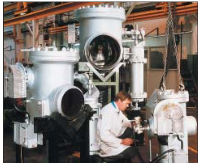
Bled steam non-return valves arranged with pneumatic power assisted closure for turbine protection.
