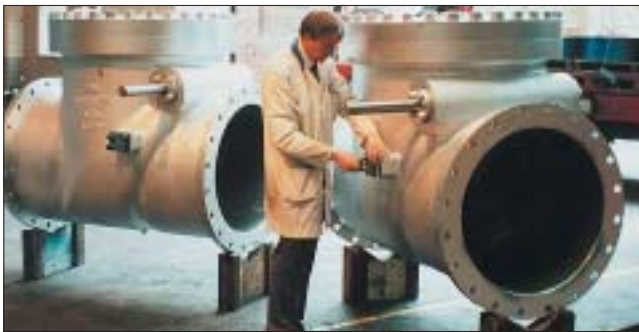
Swing check valves with extended shafts to take lever mounted weights to counterbalance the valve discs.
