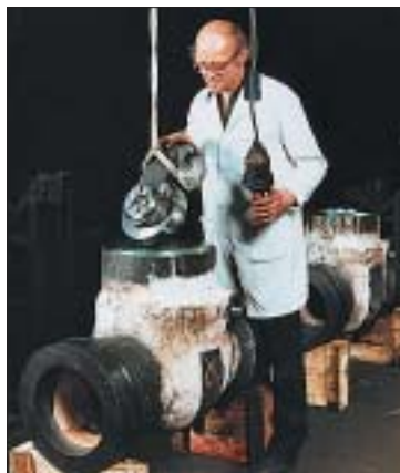
Swing check valves with extended shafts to take lever mounted weights to counterbalance the valve discs.
