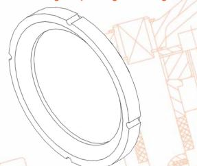
Specially designed APV seats allow equalisation of pressure in the ball cavity which reduces operating torque and increases seat life.
