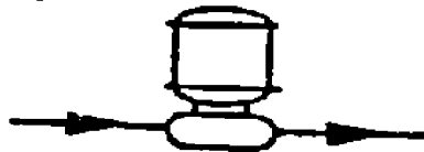
CENTRIFUGAL IN-LINE PUMP
