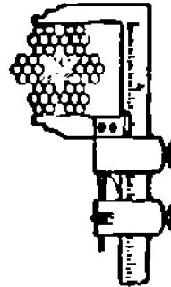
Incorrect way to measure the diameter of wire rope.
