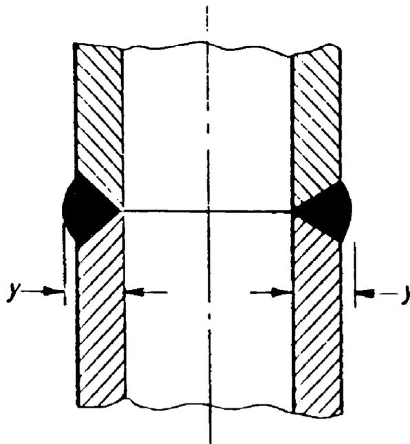
$Y$  is the thickness of metal immediately adjacent to film where there is no backing ring.
