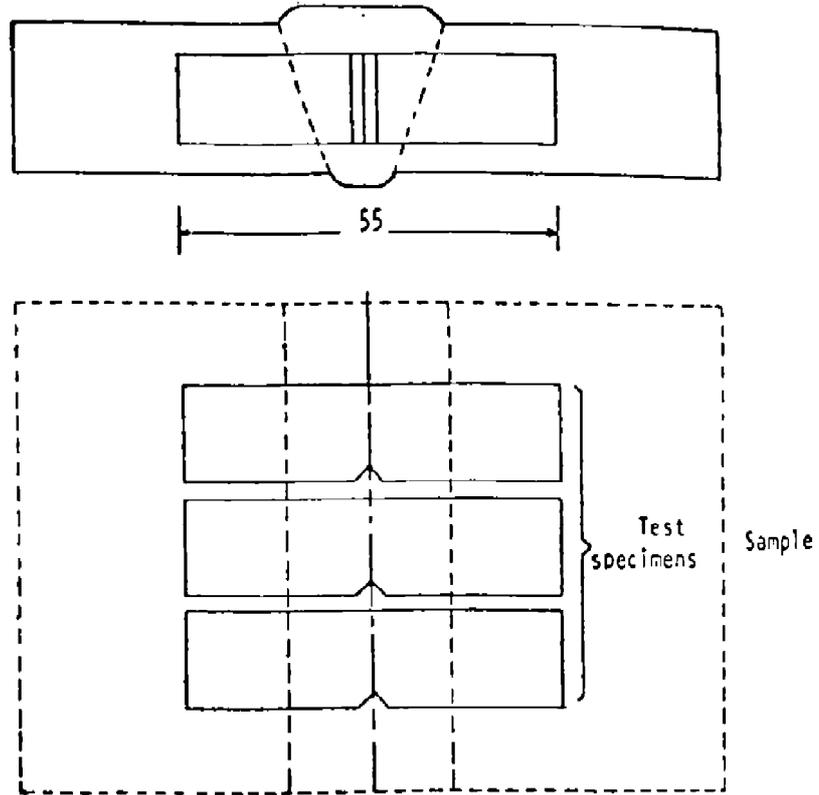
2) TEST SPECIMEN DIMENSIONS (in mm)
