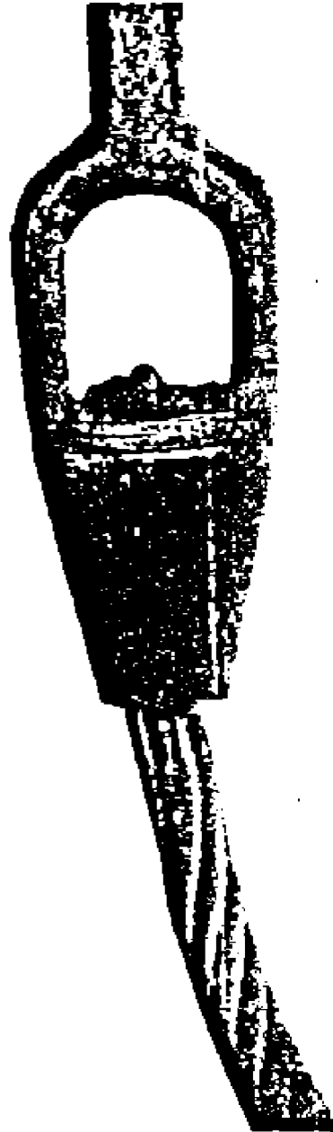
INCORRECTLY SOCKETED WIRE ROPE SHOWING LOSS OF ROPE LAY
