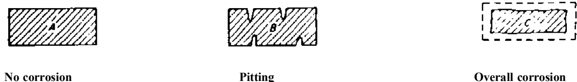
DIAGRAMMATIC REPRESENTATION OF PITTING CORROSION AS AN INTERMEDIATE STAGE
