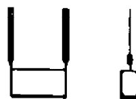
Type 3. Painter's cradles on fibre or wire ropes
