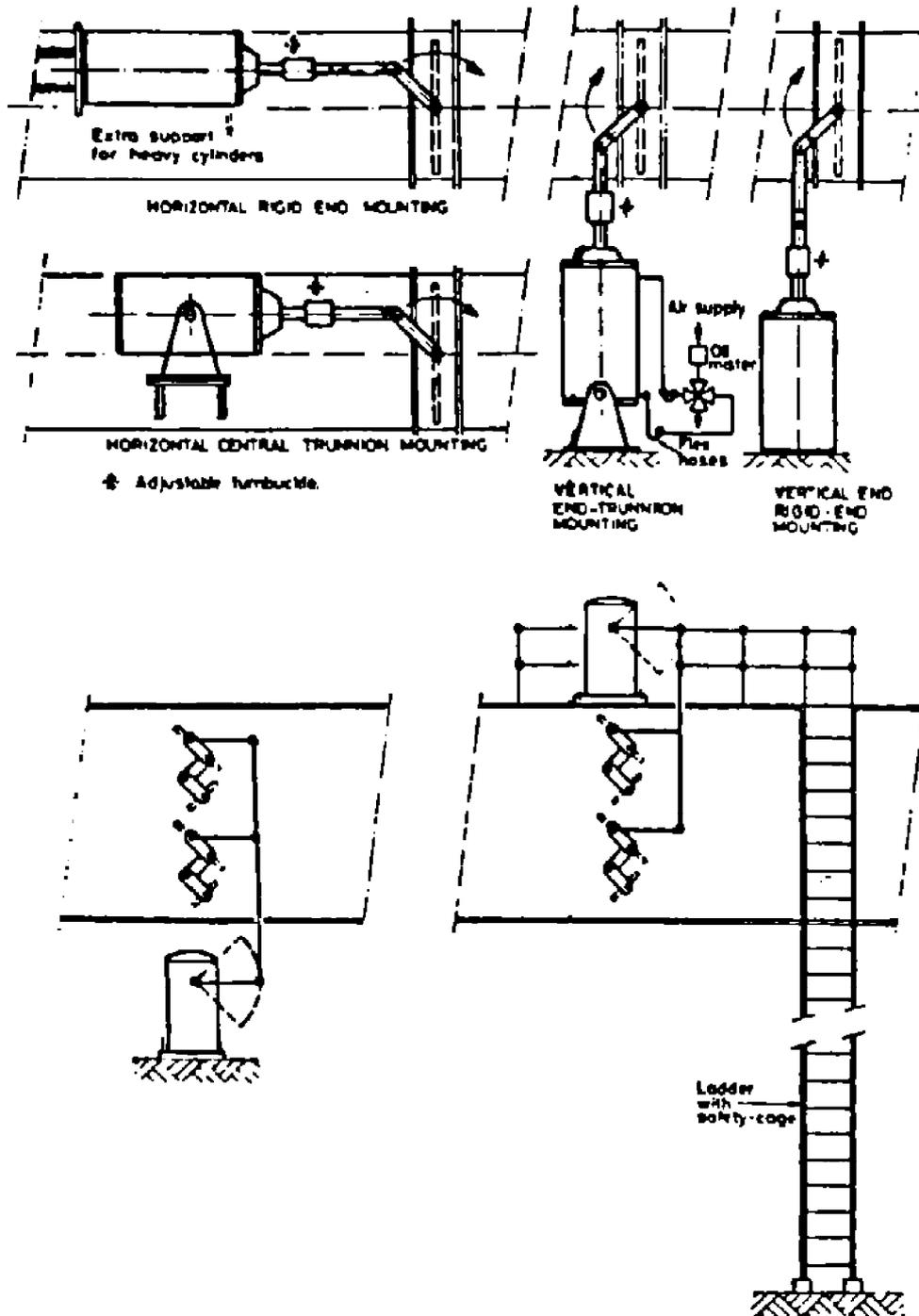
INSTALLATION OF PNEUMATIC CYLINDER ACTUATORS
