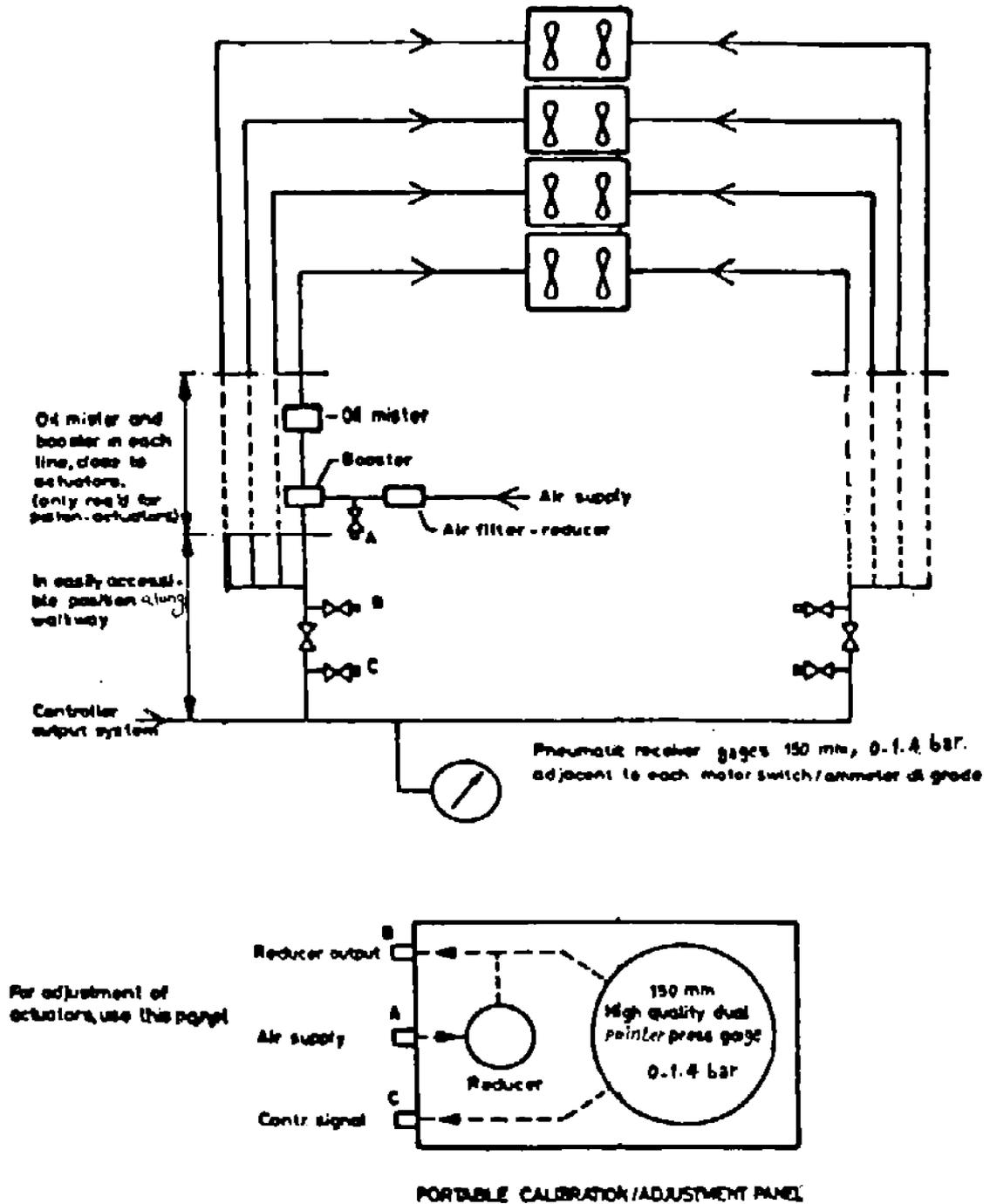
TYPICAL AIR PIPING FOR VAR. PITCH FAN ACTUATORS
