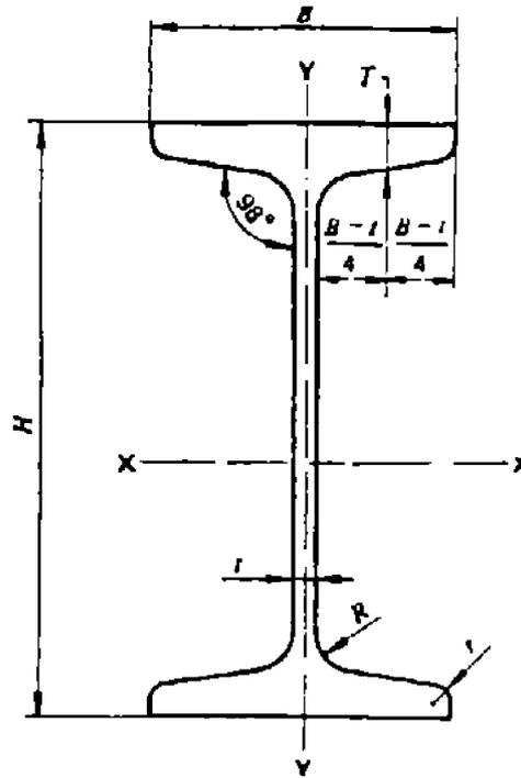
STEEL SLOPING, NARROW FLANGE BEAM SECTION
