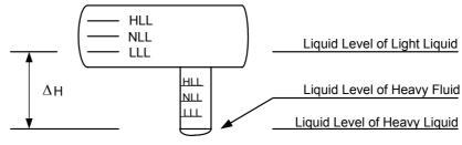
$\Delta$ H(Static Head of Light Fluid) Shall be Included in the Min. Static Head of Heavy Fluid
