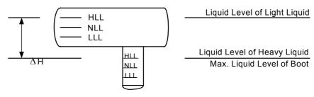
$\Delta \text{H\,Shall}$  be Included in the Max. Static Head of Heavy Fluid
