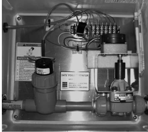
FIGURE 18.1 Example DATS® deposit monitor. (Courtesy of Bridger Scientific.)
