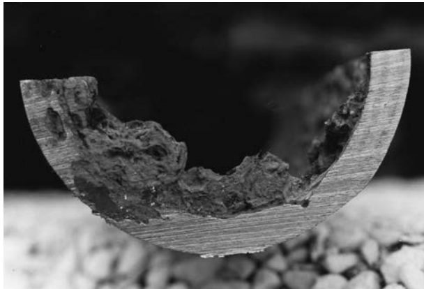
FIGURE 17.3 A pit caused by sulfate-reducing bacteria that perforated a carbon steel pipe at a weld-backing ring.
