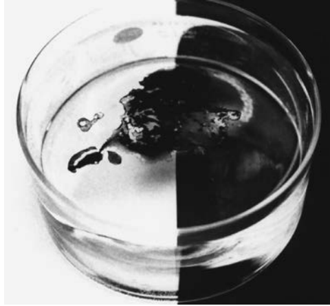
FIGURE 27.3 A few drops of oily water (w/o emulsion) when added to water will remain as a separate phase floating on the surface of the water.
