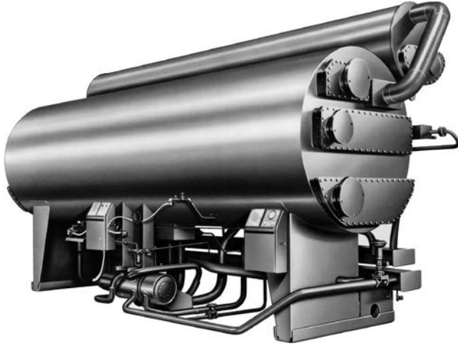
FIGURE 39.9 A steam-absorption refrigeration system, illustrating the four different chambers required for the complete cycle. (Courtesy of the Trane Company.)
