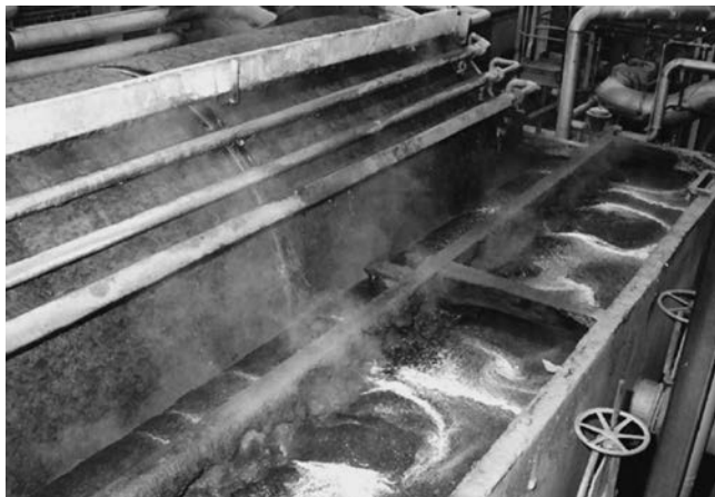
FIGURE 32.9 Photograph of a brown stock washing system.
