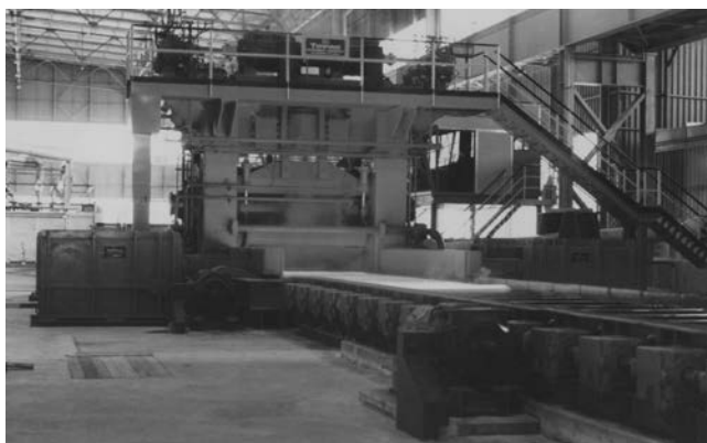
FIGURE 38.9 Hot mill rolling plate for further reduction through hot strip mill. (Courtesy of Tippins Machinery Company, Inc.)
