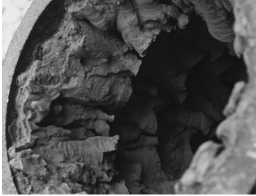
FIGURE 16.17 Example of tubercles that form long tubes in the direction of flow in a pipe.
