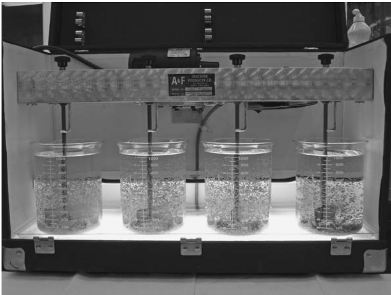
FIGURE 6.8 This type of gang stirrer is widely used for jar testing, as both a research tool and a plant control device.
