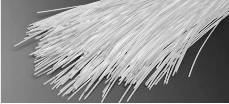
FIGURE 8.12 Hollow fiber membranes for MF and UF applications.
