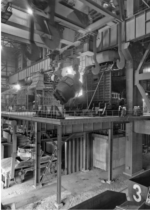
FIGURE 38.4 Hot metal is poured from the ladle into the tilted BOF as the first step in the steel making process. (Courtesy of Baumco Gesellschaft für Anlagentechnik mbH, Essen, Germany.)
