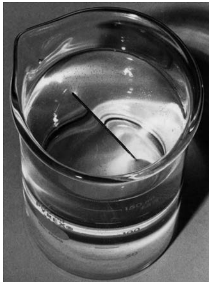
FIGURE 4.9 A steel needle, with a density about seven times that of water, can be made to float because of the high surface tension of water.
