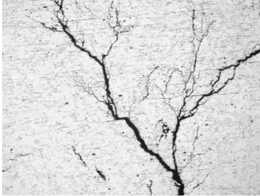
FIGURE 16.25 Stress corrosion cracking showing the typical branching of the crack.
