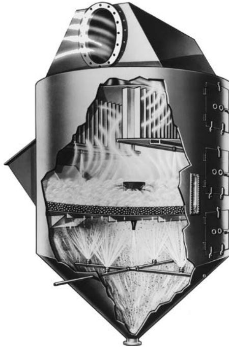
FIGURE 28.6 Moving bed scrubber using lightweight packing of spheres that continually shift, preventing plugging. (Courtesy of The Ducon Company, Inc.)
