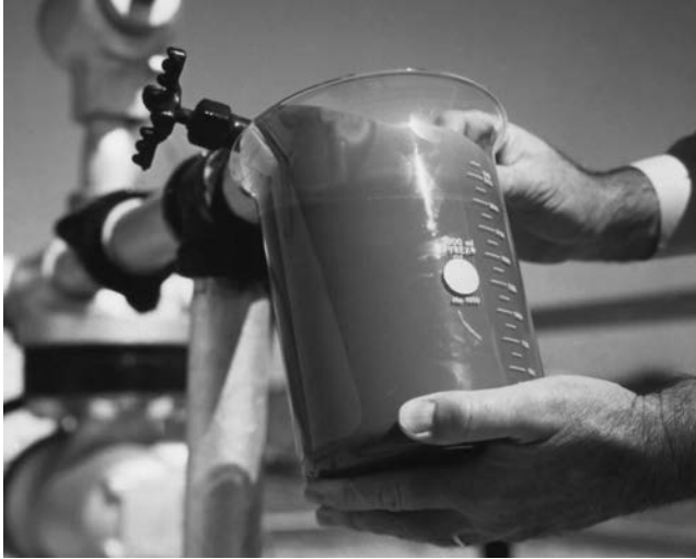
FIGURE 34.6 Oil is almost always produced as an emulsion, very different in appearance from finished oil products.
