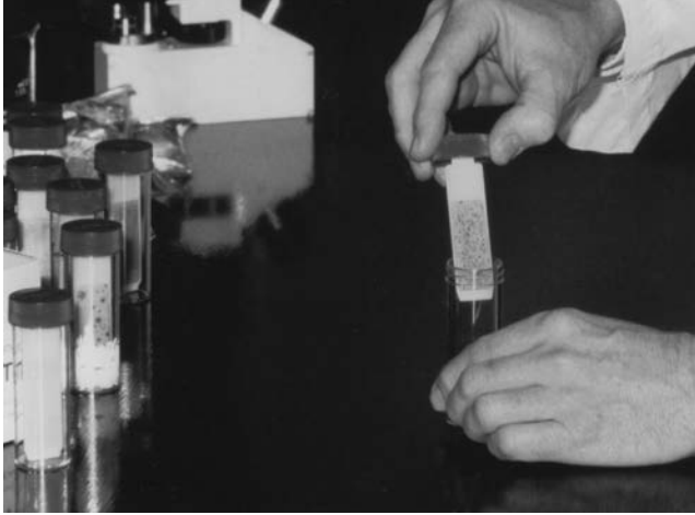
FIGURE 18.17 Microbes are collected and cultured by pretreated elements, which are easily incubated in the sampling container. (Courtesy Millipore Corporation.)
