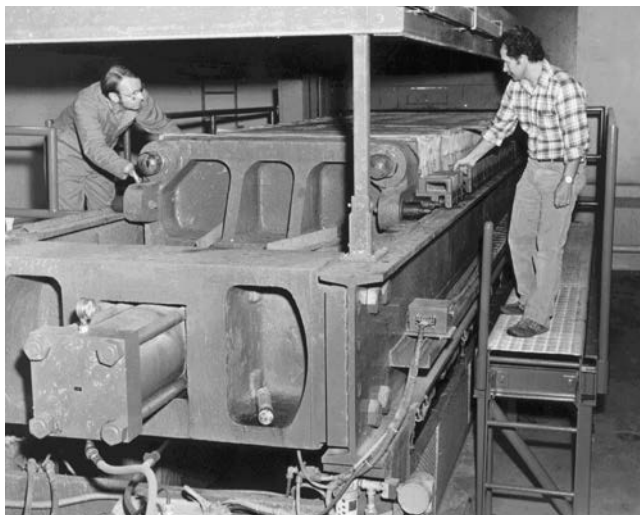
FIGURE 26.10 Plate-and-frame press dewatering sewage plant sludge.
