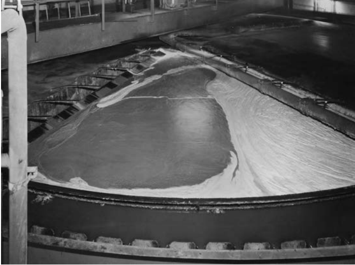
FIGURE 27.10 The float produced by DAF of an oily effluent (o/w) emulsion. (Courtesy of Infilco Degremont Inc.)
