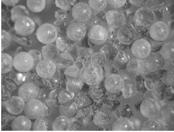
FIGURE 7.43 Organically fouled SBA resin before a brine squeeze.
