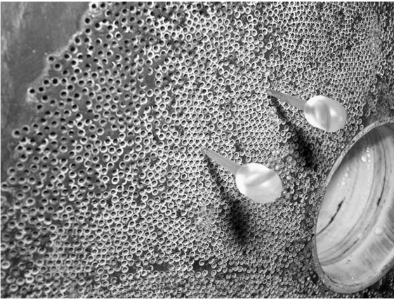
FIGURE 8.22 Pinning broken fibers identified during air integrity testing.
