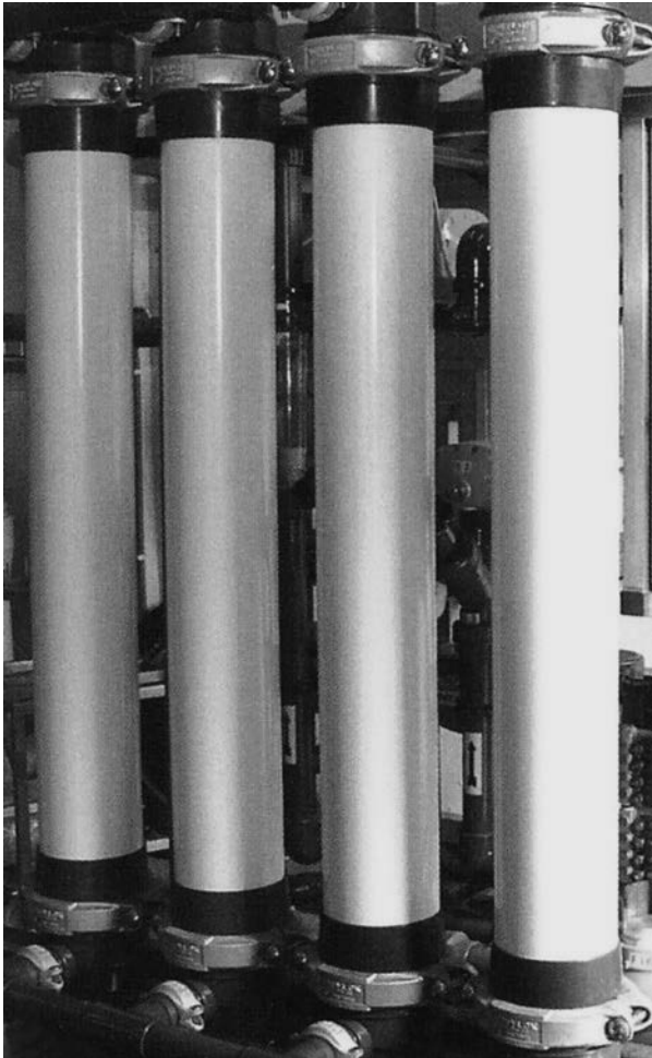
FIGURE 8.15 Canister-type hollow fiber membrane modules for MF and UF applications.
