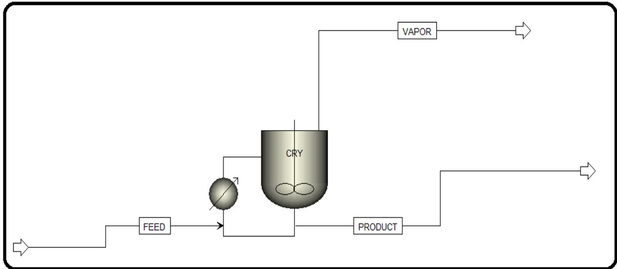
5. Figure 14.29 shows the feed stream properties in terms of  $P$ ,  $T$ , and compositional flowrate. There will be no need for PSD specification because the feed stream is a saturated aqueous KCl solution entering at the maximum solubility, which is 35 g KCl/100 g water (amounts to KCl mass fraction of 0.26).
