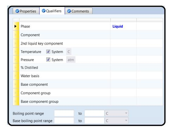
We must now add the "TXPORT" property set to the stream table that is shown in the process flowsheet. While "Simulation" environment is the active mode and using "Navigation" pane, go to "Setup" | "Report Options" | "Stream" tab form and click on the "Property Sets" button. Doing so will open up the window shown in Figure 3.12.
