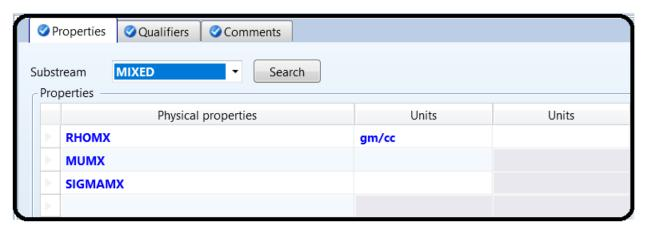
Select the last row (or record) in the first column that is currently blank. In doing so, you will be presented with a scrolling window of physical properties that Aspen Plus can calculate for the user. Scroll down until you find "DMX" (Diffusivity of a mixture), which is the variable for diffusivity in Aspen Plus. You will notice that a description of each physical property appears as you hover the mouse over the variable name.
