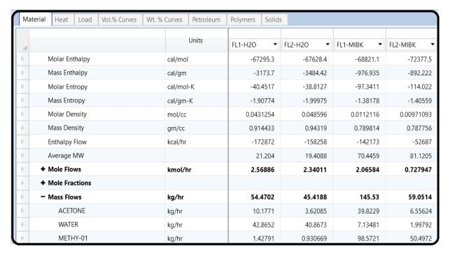
NOTE #0: The simulation and design specification results in this chapter will be subject to how we let Aspen Plus calculate binary interaction parameters among the three components. So, be sure that, under "Methods" | "Parameters" | "Binary Interaction" | "NRTL-1" sheet, the source for each of the three columns is selected as "APV88 VLE-IG" not "R-PCES". See Chapter 3 on how to set the source as "APV88 VLE-IG". Keep in mindthat this does not advocate using "APV88
