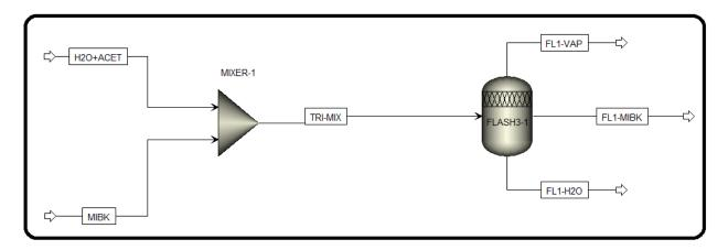
To hook "TRI-MIX" stream to the flash separator right-click on "TRI-MIX" stream, out of "MIXER-1". Select "Reconnect" menu→"Reconnect Destination" submenu and attach this stream to the
